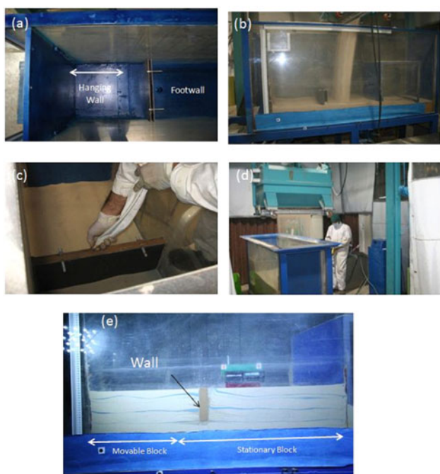
Fig. 5 1 g model test (a) putting two steel plates in the box; (b) sand pluviation up to 5 cm; (c) the space between two plates filled with clay (clay height is 15 cm); (d) filling the box with sand; and (e) sand and clay wall after two steel plates carefully extracted
